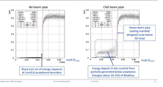
During the workshop in Annecy Mogens Dam highlights the weakness of the ellipto-conical chamber design with the copper cooling
