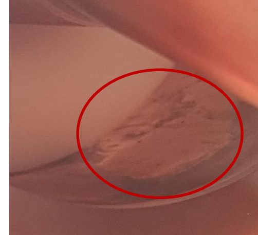
Severe loss of Cu near vacuum port. Edges are sharp...
