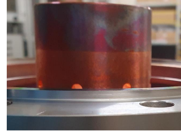
Discoloration band on inner conductor
