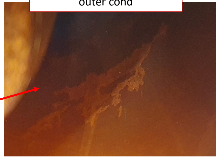
A band of arcs/MP on outer cond
