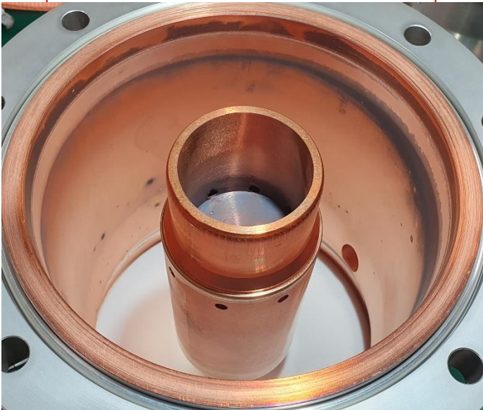
Marks on outer cond. – heat inside inner cond.
