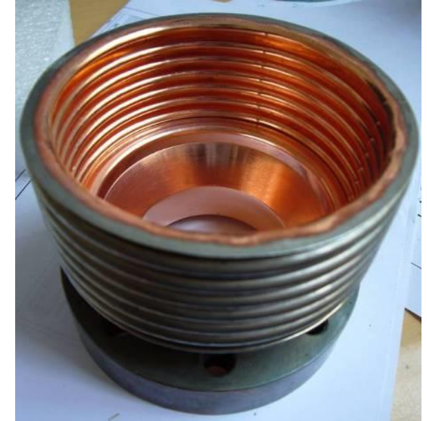
The warm ceramic window of waveguide type
