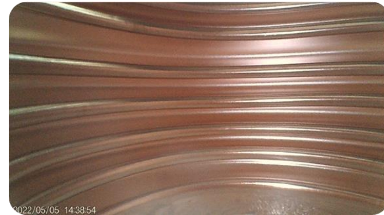
Copper-plated inner surface of bellows after continuous drawing.
