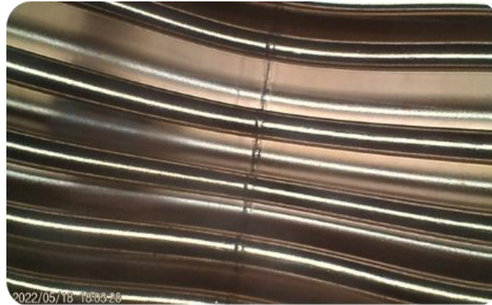
Liquid nitrogen thermal shock test (liquid nitrogen to air) - one cycle
