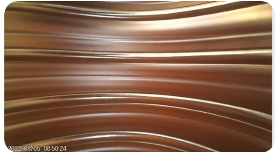
Copper-plated inner surface of bellows after vacuum heat treatment
