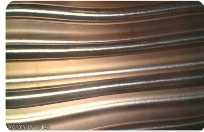
Liquid nitrogen thermal shock test (liquid nitrogen to warm water) - three cycles
