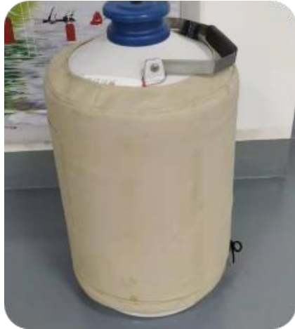
Liquid nitrogen tank
