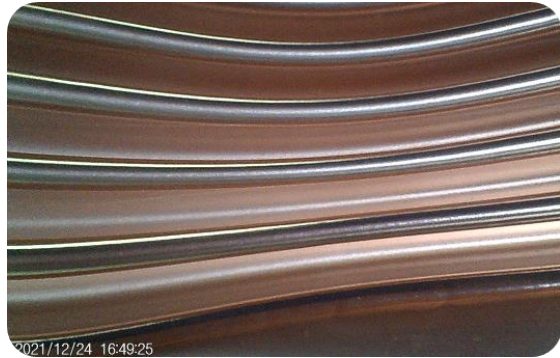
bellows copper plating (inner surface)
