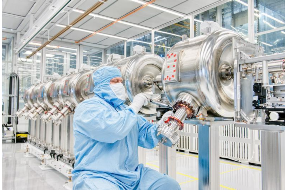
Installing vacuum parts of SSR couplers
