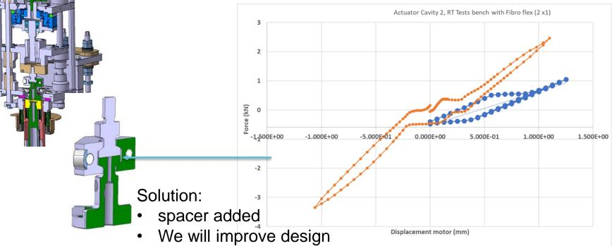
Removed the actuator support + <u>springs</u>. The actuator now "sits" completely on cavity. This to reduce the restraints on bearings + bonus: no more interference with waveguide or cable FPC
