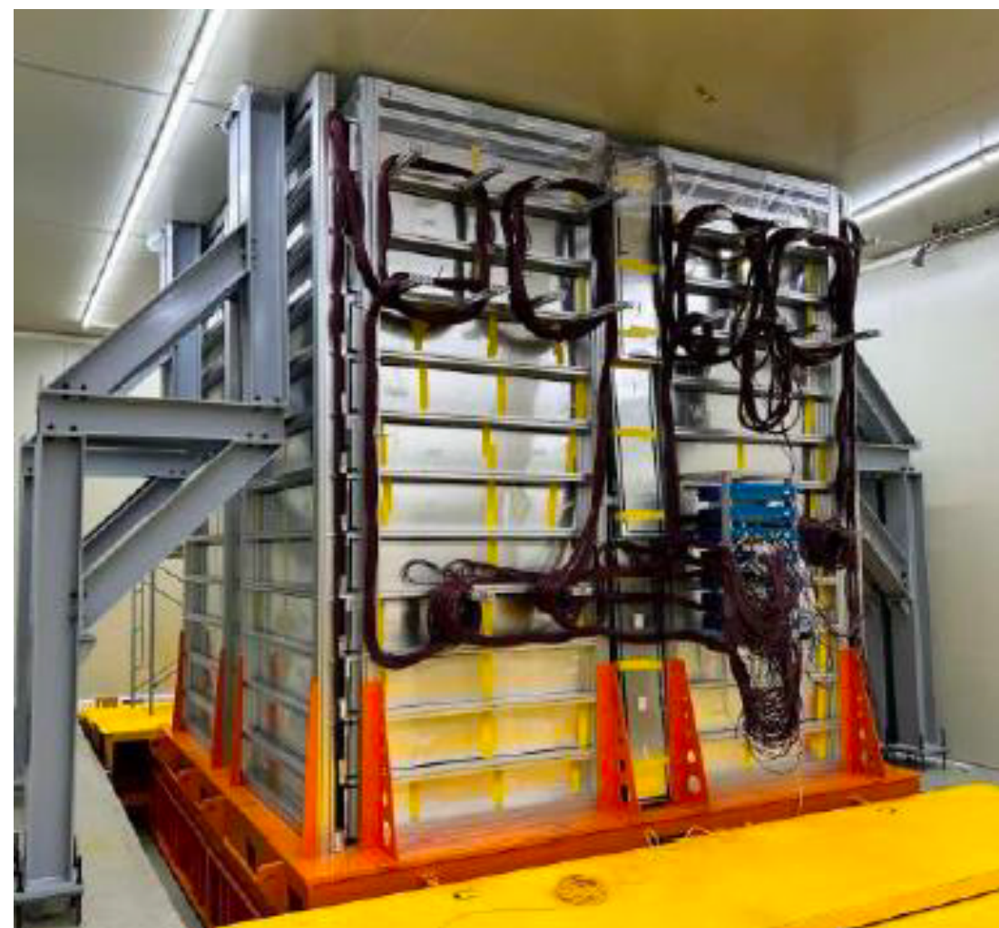
← Bottom plastic scintillator: 130 modules × 2 PS panels × (WLS fibers+2 SiPM)
