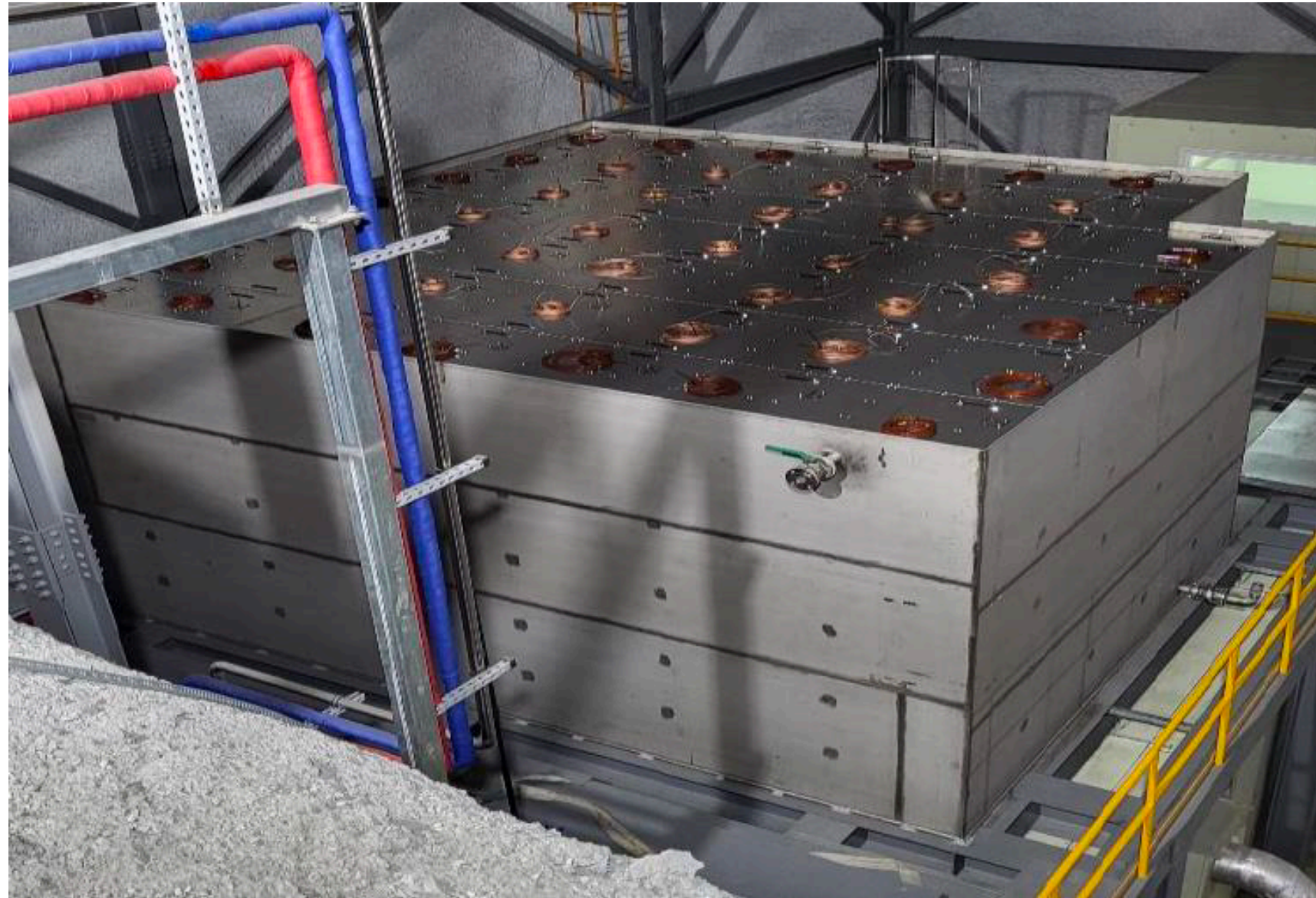
↑ Water Cherenkov at the top: 70 cm thick (60 tonnes), 8, 10 inch PMTs
