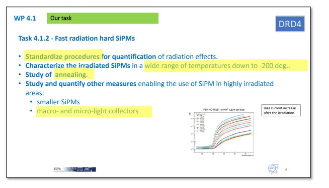
Mostly focused on **silicon technology** to improve the sensor properties (dark counts, efficiency, fill factor, time res., etc). Aiming at small-scale novel devices (often single-channel) in collaboration with foundries. As well as close integration with readout electronics (2.5D/3D sensor).
