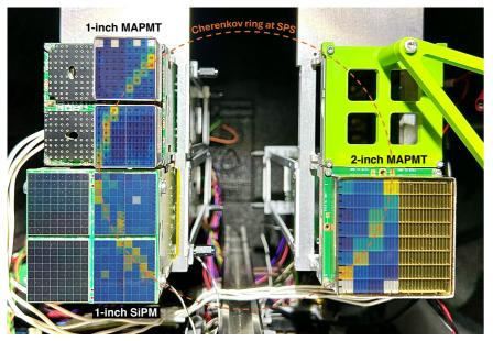
Hit maps, from recorded data, of the Cherenkov ring arcs superimposed on the active area read out by the FastIC chain.
