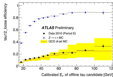
The histogram to the left shows a comparison of  $Z \rightarrow \tau\tau$  signal MC to QCD di-jet background for the tau12\_loose HLT chain. After the application of a loose di-jet event selection, the trigger efficiency for data taken in 2010 agrees very well with the QCD background sample after applying a tight offline tau selection. The uncertainties shown include statistics only.
