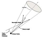
The SV0 tagging algorithm relies on reconstructed secondary vertices from the tracks associated to jets.
