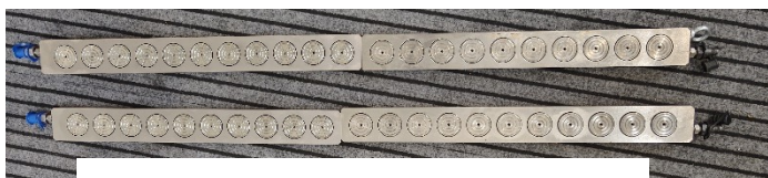
Hydraulic pre-loading system
