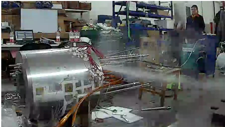
Leaking bladder during the assembly of LPF1
