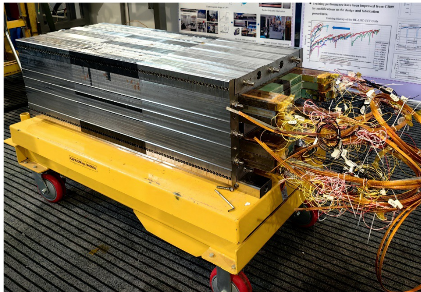
coils assembled with the H-pad & V-pad
