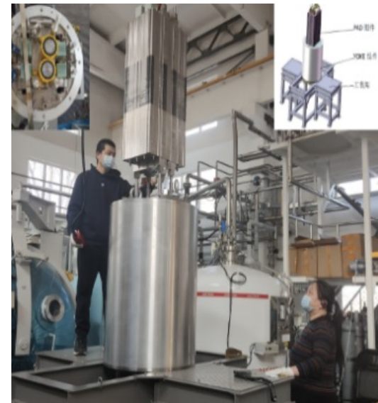
Vertically assemble the Coil & Pad and yoke & shell
