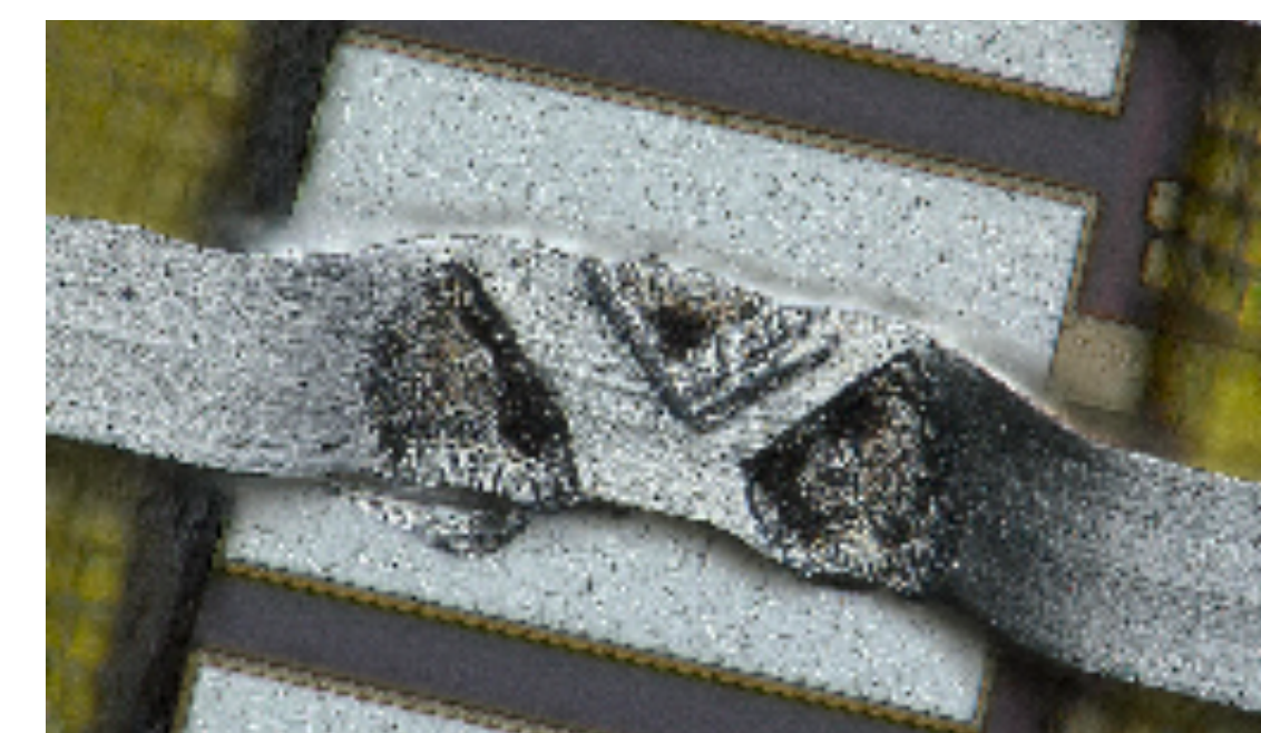
SpTA-Bond connection: bond pads size 200 x 100 µm 2
