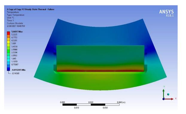
Initial FEA thermal simulation of the PLR ring with a linear triplet module - the mechanical structure used in the calculation is the same as shown in the previous two figures. The geometry and heat-flow impedances should be fairly accurately modelled. This figure is for a "normal operation" scenario for the Shunt-LDOs. The  $\Delta T \approx 5^{\circ}$  is well within requirements
