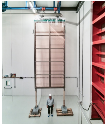
The DUNE anode wireplane assembly
