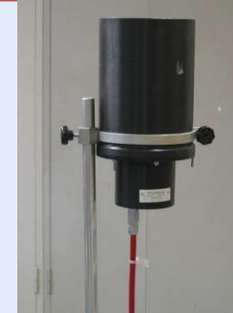
Air filled ionization chamber
