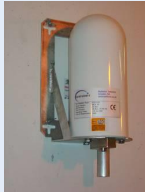
Gas filled, high pressure ionization chamber
