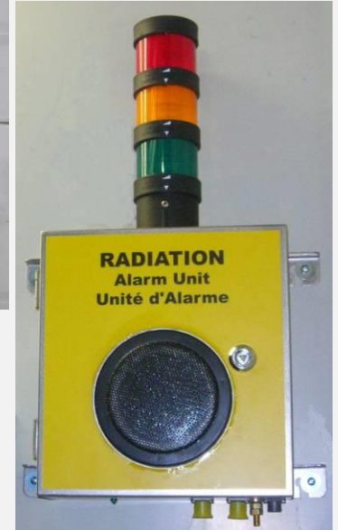
Radiation Alarm Unit (RAMSES)
