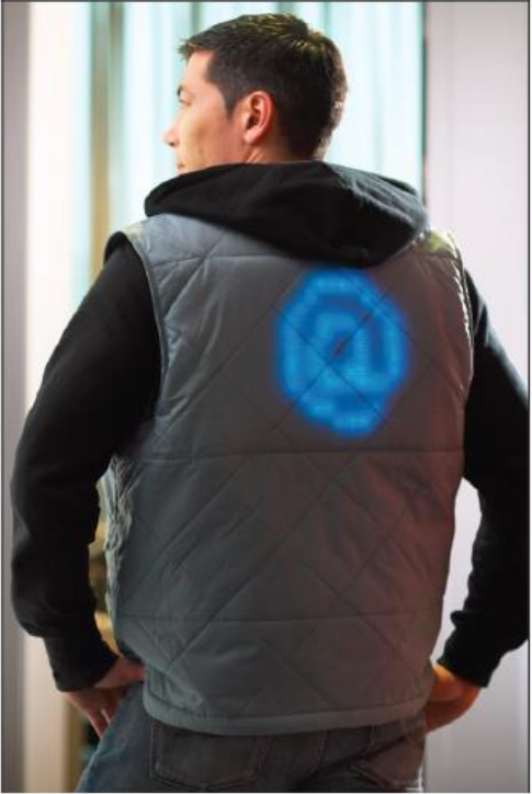
Lumalive textile from Philips features flexible arrays of colored LED fully integrated to the clothes
