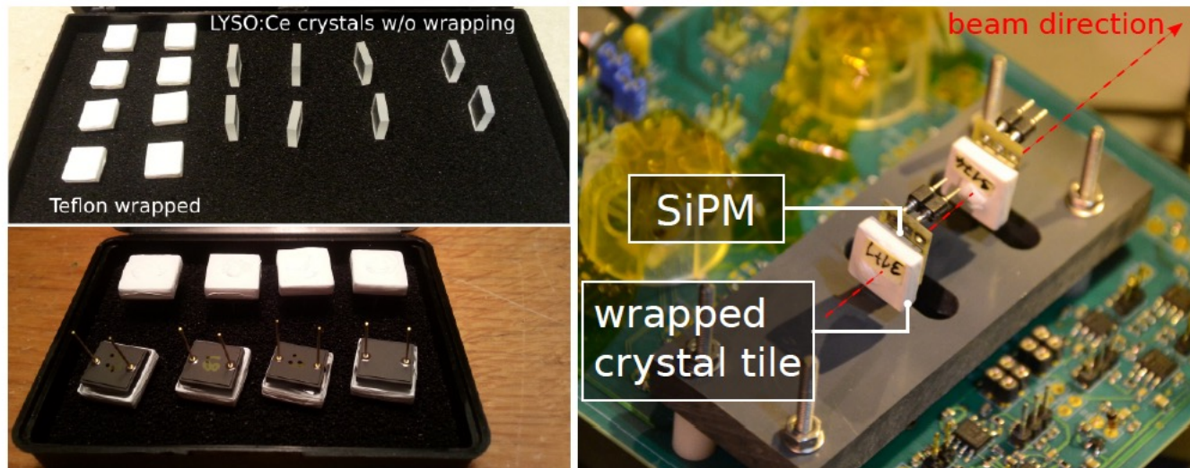
Figure 2.4: Top left: Set of 11 \times 11 \times 3 \text{ mm}^3 LYSO:Ce crystals with depolished lateral faces, before and after Teflon wrapping. Bottom left: 6 \times 6 \text{ mm}^2 HPK SiPMs glued on LYSO crystals. Right: Crystal+SiPM sensors plugged on the NINO board used for test beam studies.
