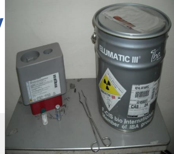
Molybdenum technetium generator {}^{99}\text{Mo}/{}^{99\text{m}}\text{Tc}
