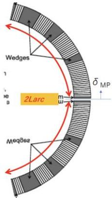
$\delta_{MP}^{sim}$  was estimated from the measured coil-size asymmetry, assuming no friction between the cables and collar. The measured skew quadrupole is largest in MBXF3, but still within 5 units
