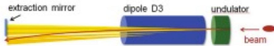
Figure 1: Sketch of the BSRT light sources.
