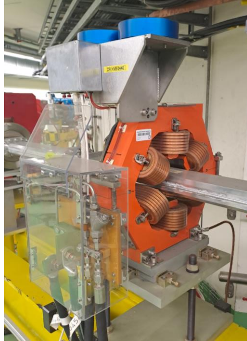
Renewed quads and sextupoles with large aperture
