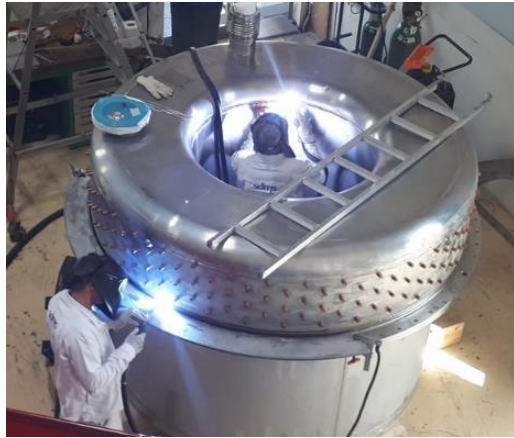
Welding of the He vessel
