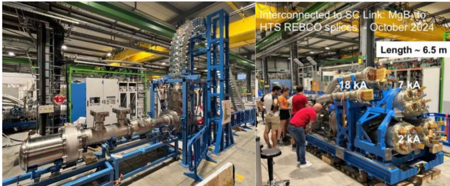
Full-size HL-LHC superconducting link prototype system successfully tested in March 2024 (transferred up to ~ 94 kA in DC mode)
