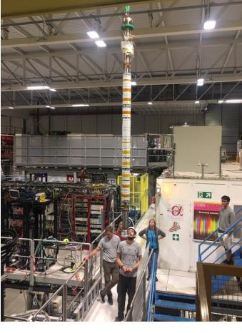
1 T 50 cm bore, 3m solenoid from Bilfinger Sumitomo cryocoolers
