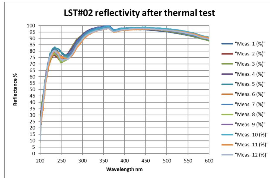
Reflectivity measurement carried out on 12 points distributed along three diagonals on prototype
