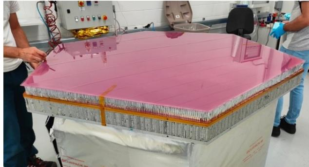
*Sandwich structure on the mould*
