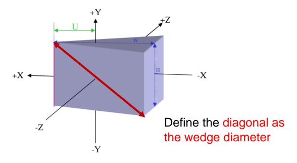
Scale the window thickness by diameter with the thickness in MICE. Be is window material (low atomic number).
