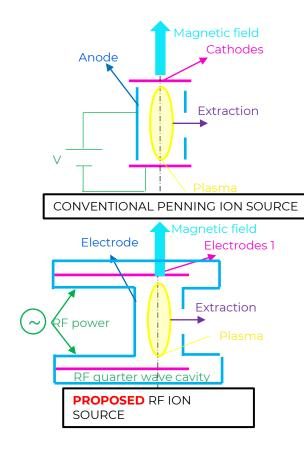
A new concept of internal ion source based on RF for cyclotrons: Change DC voltage of conventional Penning ion source to a RF voltage
