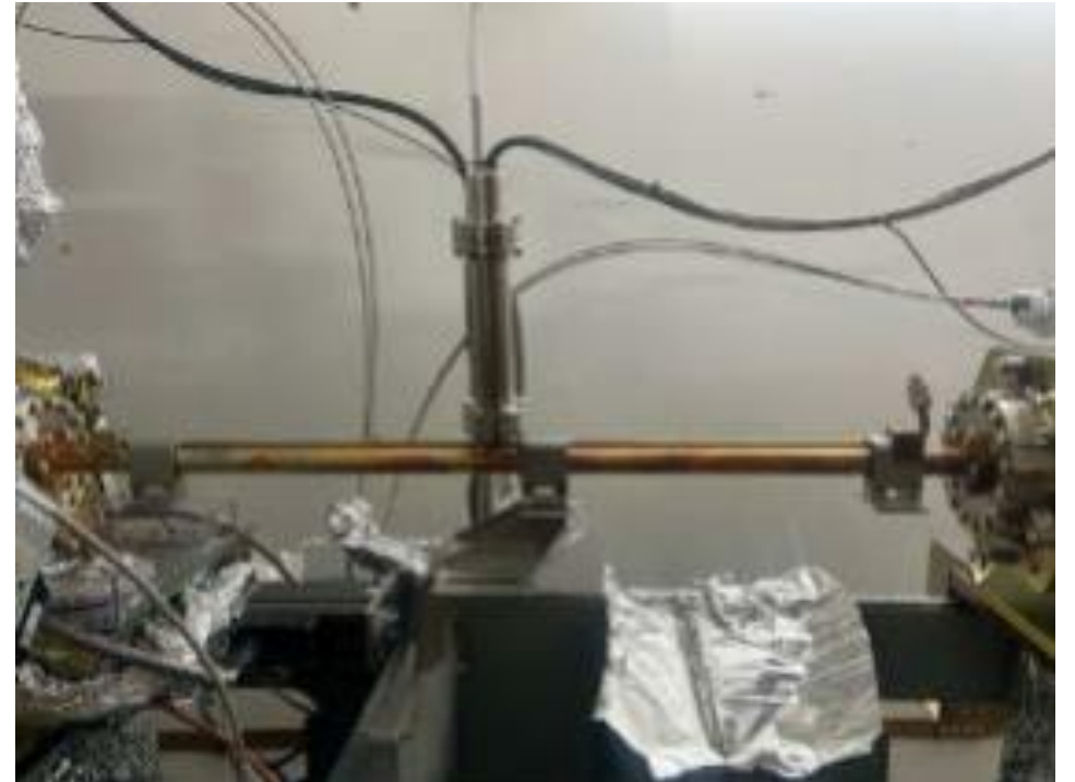
The TiZrV NEG coated copper sample with ID = 20 mm and L = 1.0 m installed in the SR beamline at DLS
