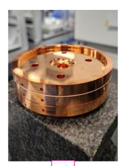
• The alignment and flatness of the structure were kept as expected after the cycle with the 40kg on top.
