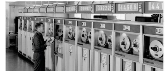
The tape-unit reel-display system (RDS) shown mounted over tape units in the 6600 computing complex, in 1965.
