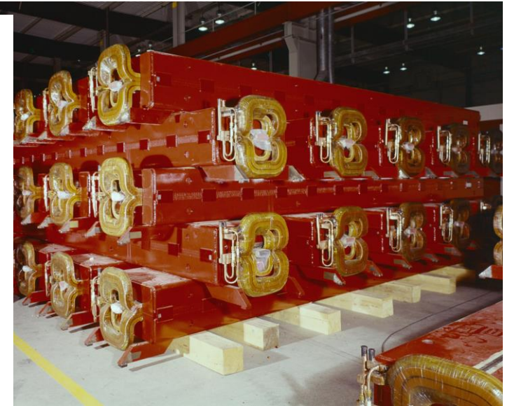
SPS main bending. 2.0 T, 5.8 kA
