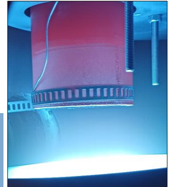
HiPIMS glow discharge during a quadrupolar sample coating
