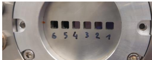
Window #1 \text{Si}_3\text{N}_4 – spots 5 & 6 broken
