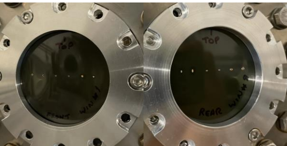
Gauged film shows focused beam upstream and divergence downstream
