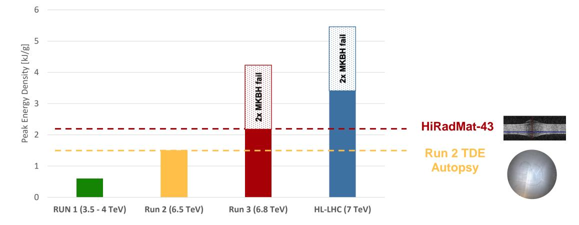
> Run 2 TDE Autopsy  $\rightarrow$  No out-of-plane deformation, minor darkening on some disks
