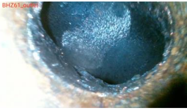
Brazing of Cu block to SS insert
