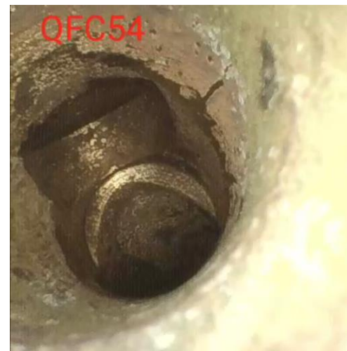
Cu erosion due to high water speed (8 to 14 m/s)
