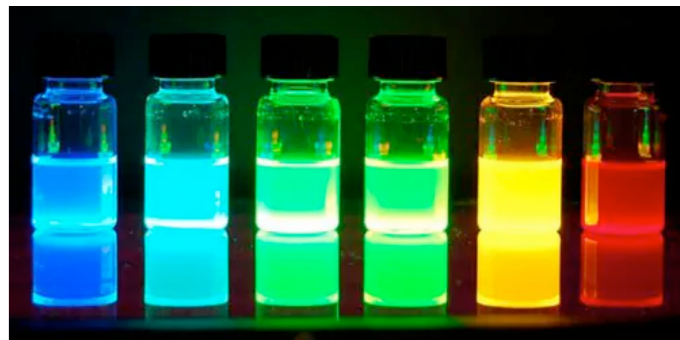
Photoluminescence of alloyed CdS_xSe_{1-x}/ZnS quantum dots of 6 nm diameter. The material emits different color of light by tuning the composition.
