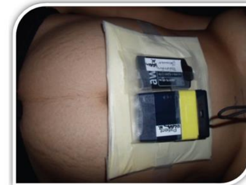
Figure 1.24: Foetus dosimetry during radiotherapy of a pregnant woman with C-ions at HIT.
