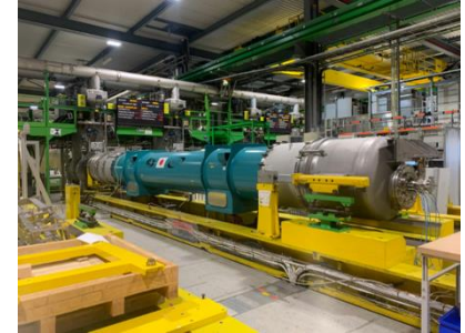
KEK D1 prototype under test at CERN.
