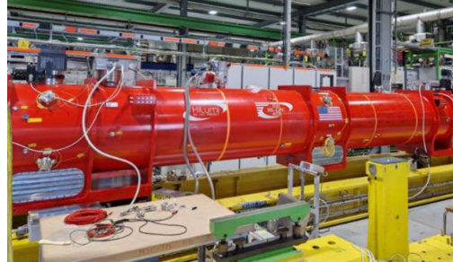
First US inner triplet cryoassembly connected to CERN test station
