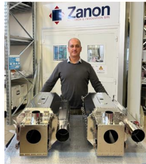
Magnetic shields & helium tank materials ready for first two bare RFD cavities (Zanon, IT)
