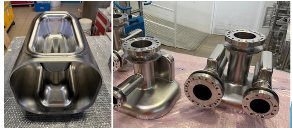
Some Components of Series #3 and #4 ready for trim-tuning
