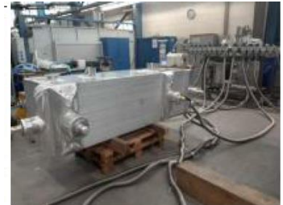
PFHE test at Linde premises
