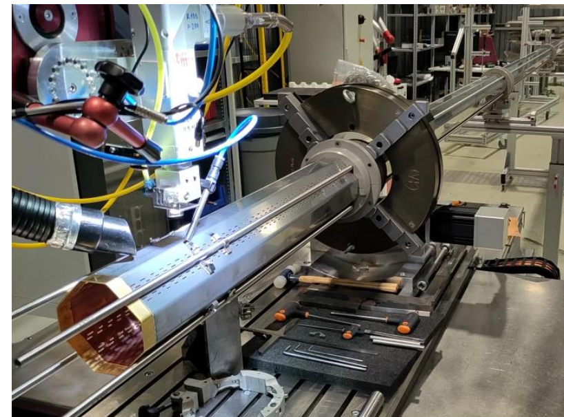
Cooling tube welding
