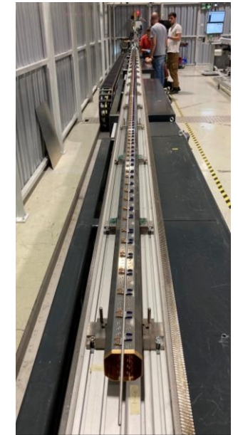
D2 cooling tubes tooling
