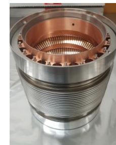
PIM with Deformable RF bridge Completed (30) First PIM assembled
