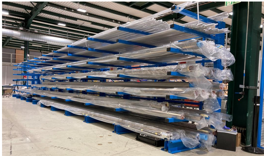
All (39+12) BS tubes butt welded and ready for assembly
