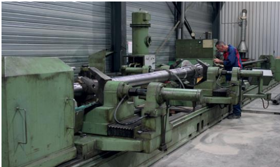
Honing of cold bores
