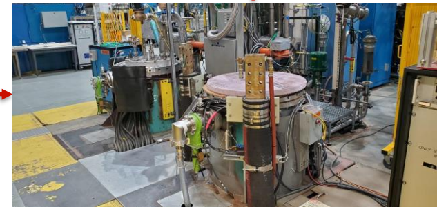
Magnet in Test Dewar with Field Measurement Probe
