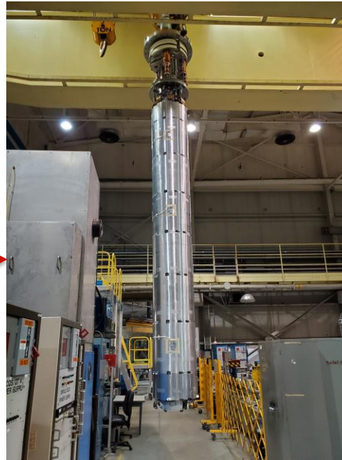
Prepared magnet with all power and instrumentation connection transported to test Dewar
