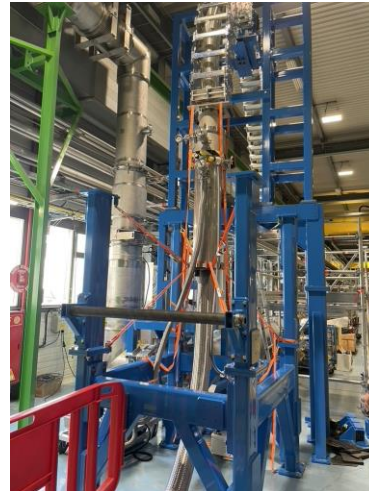
Leak Tightness of the SC Link + DFHX
