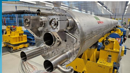
X lines positioning and welding copper rings
