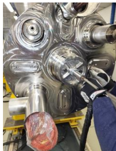
V line alignment and gas protection system preventing cbt deformations
