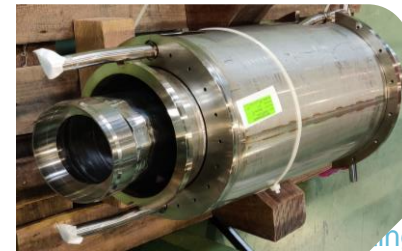
Diode connection on SC busbar and NbTi-NbTi Splices (mock-up)
