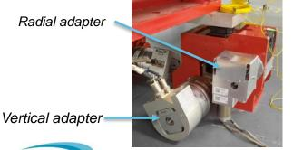
Adjustment solutions for a light component (< 2 tons)
