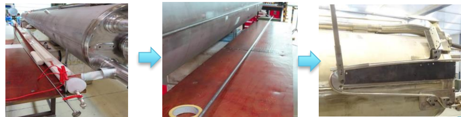
Test of wires in water (steps 500 V/30 s – 1000 V/120s – 2000 V/120s) + Drying
