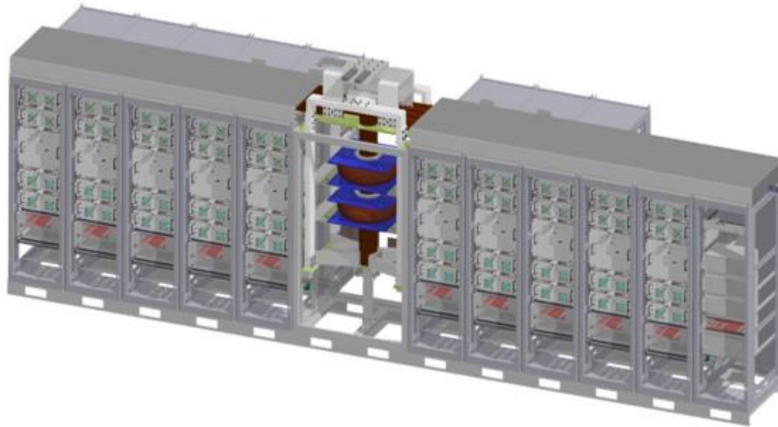
18kA Power Converter of RQX circuit
