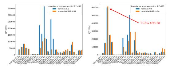
In y the IR3 collimator TCSG.4R3.B1 (horizontal secondary) dominates the impedance. Therefore, the impedance reduction coming from the IR7 is overall less effective.
