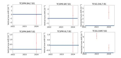
Again positive horizontal tune-shifts for the vertical collimators.
