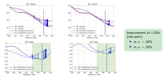
It is ok to have less improvement in y because with the standard optics x is the most unstable plane.
