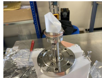
New SR extraction mirror and new extraction tank in IR4L
